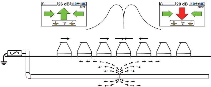
(Note that the A-frame is not shown connected to the receiver so as to simplify the diagram)
