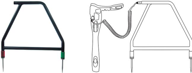
The vLoc3 series A-frame accessory is used to detect ground faults on pipes and cables. In the case of pipes, the faults consist of coating defects. In the case of cables, faults are usually caused by insulation damage allowing the metallic sheath (or internal conductor) to become in contact with the ground.
